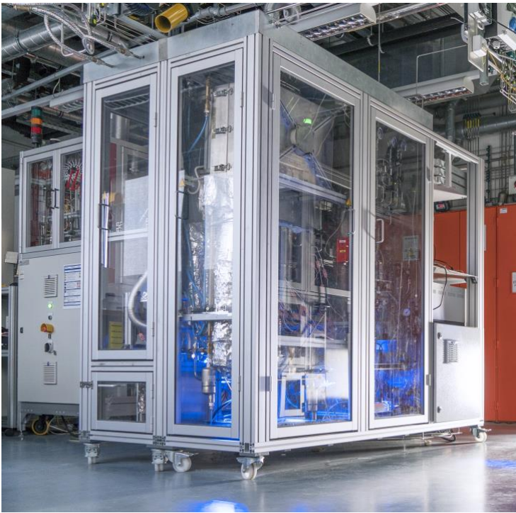
Figure 1: Lab-scale integrated Power-to-Liquid plant.
